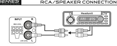
Der US OB ACTIVE has RCA inputs, which are connected by RCA cable with the preamp outputs of the control unit (Headunit, MP3 player, iPhone, iPad). If this is not possible (usually with an original radio, OEM), the loudspeaker outputs of the Headunit can be connected directly to the HIGH-LEVEL inputs and the switch can be set to "Auto Power". The amplifier turns on automatically when a signal is present.
