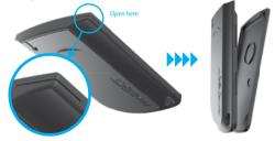
Carefully open the cover of the tag's battery compartment. Extract discharged battery and insert a new one keeping in mind the correct polarity. Replacing a battery will not cause a loss of tag code information, as authorization data is stored in the non-volatile memory of the MCU. Carefully close the cover of the tag's battery compartment. All elements of construction should be rigidly locked in places. If it is so, the tag can be operated as usually.
