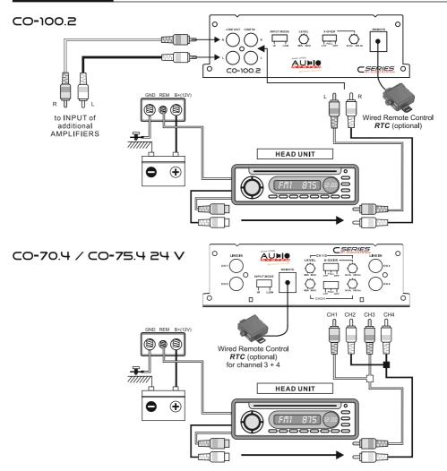
The CSERIES amplifier offers RCA-Inputs, which are connected through cinch cables with the preamplifier-outputs of the head unit. If the head unit (OEM-RADIO) has no RCA-Output, than it is possible to connect the speaker output direct to RCA/Cinch-Input of the amplifier.
