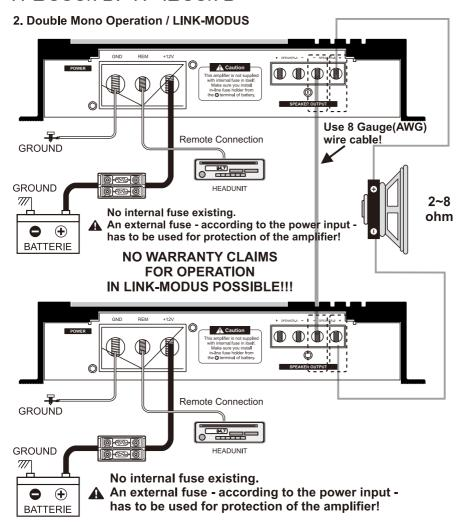
In a dual-mono operation of 2 X H-3000.1 D / 2 X H-4500.1 D assumes the "master amplifier 'total control of the" slave power amp ". The positive (+) terminal of the subwoofer must be connected to the positive terminal of the "Master amplifier". The negative (-) terminal of the woofer to the positive (+) of the "slave power amp". When dual-mono operation of two H-3000.1 D / H-4500.1 D amplifiers, immense power is produced. Please make sure that the connected speakers are suitable for this.
