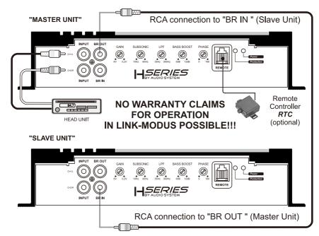
The H SERIES amplifier offers RCA-Inputs, which are connected through cinch cables with the preamplifier-outputs of the head unit. At the "BR OUT"-RCA it's possible create a Master-Slave-Modus with a second H-3000.1 D or a second H-4500.1 D.
