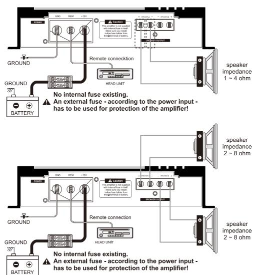
Please note that the H-3000.1 D + H-4500.1 D are pure mono amplifier. When connecting 2 speakers or a dual voice coil subwoofer, the speakers (voice coils) are connected in parallel. It should be noted that each coil has not less than 2 ohms. The total impedance is then 1 ohm.
