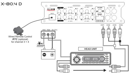
The X SERIES amplifier offers RCA-Inputs, which are connected through cinch cables with the preamplifier-outputs of the head unit. If the head unit (OEM-RADIO) has no RCA-Output, than it is possible to connect the speaker output direct to RCA/Cinch-Input. Important: the Gain-Controller has to be adjusted to minimum, then carfully turn up the volume. Input Mode has to be switched on "HI". If signal is presented, the amplifier automacally turns on.
