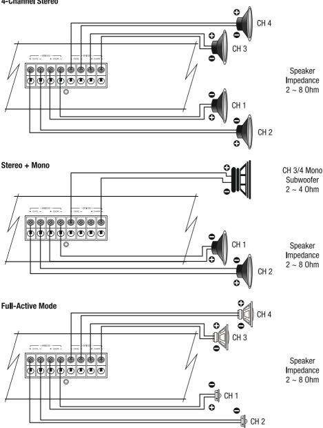
At Full-Acitve Mode the high pass filter and low pass filter have to be adjusted confirming to the used midrange speaker and tweeter. **Therefore contact you specialist dealer.**
