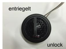
The attached lock/unlock tool is design to fit in the holes of the tweeter-grille. Turning the tweeter to the left will lock the tweeter into the housing, turning to the right will unlock the tweeter.
